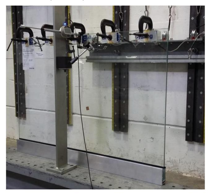
Typical arrangement for application of horizontal uniformly distributed line loading assembly
